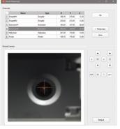
• By automatically recognizing the surface height value of bioware and fine-tuning the X / Y coordinates between the nozzles used for output, highly stable extrusion 3D Printing can be achieved.
